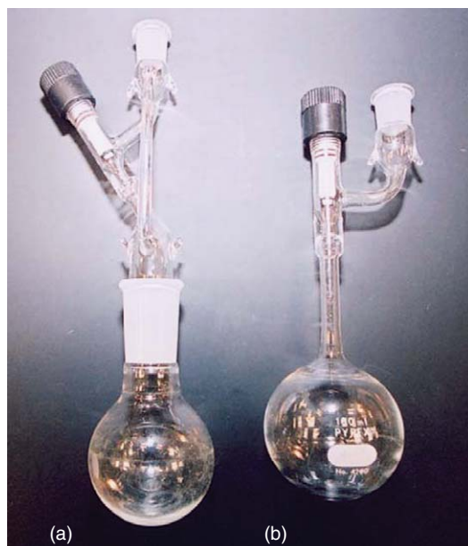
Figure 5 (a) Example of a standard taper round bottom flask and its adaptor for use on a high vacuum line. (b) Example of a one-piece flask designed for use on a high vacuum line.
