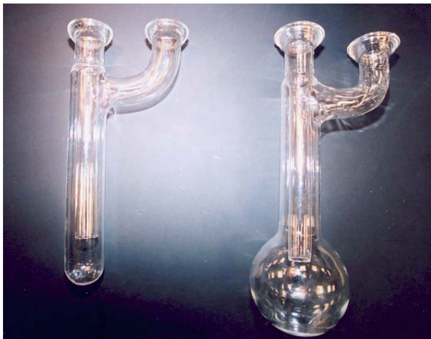
Figure 4 Solvent traps can be designed to handle both small (left) and large (right) amounts of solvent.
