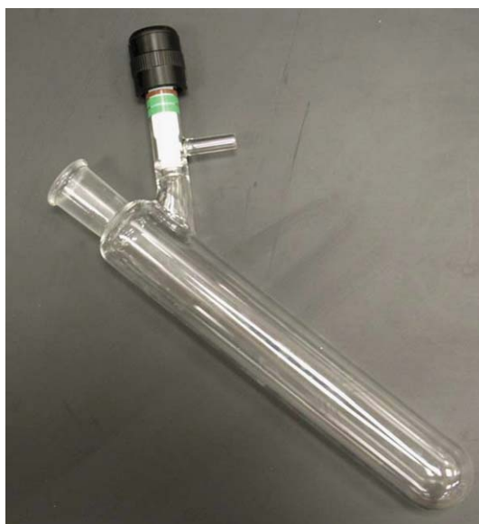
Figure 7 A commercially available Schlenk tube containing a PTFE valve. The valve, tube, and ground-glass joint sizes may vary.
