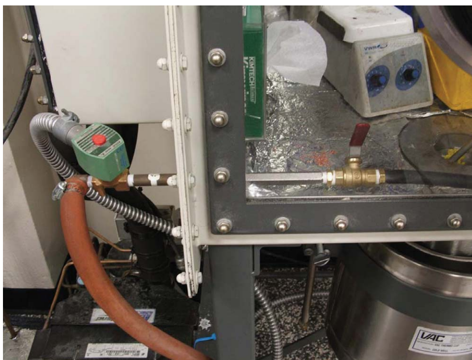
Figure 21 Picture of a pipe fitting adapted for vacuum filtration use inside a glovebox. The solenoid valve controls an opening to a vacuum source through a foot switch (not shown).
