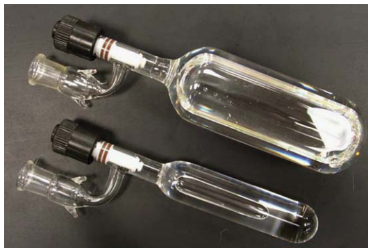
Figure 17 Air-free ampoules used for deuterated solvent storage and transfer.
