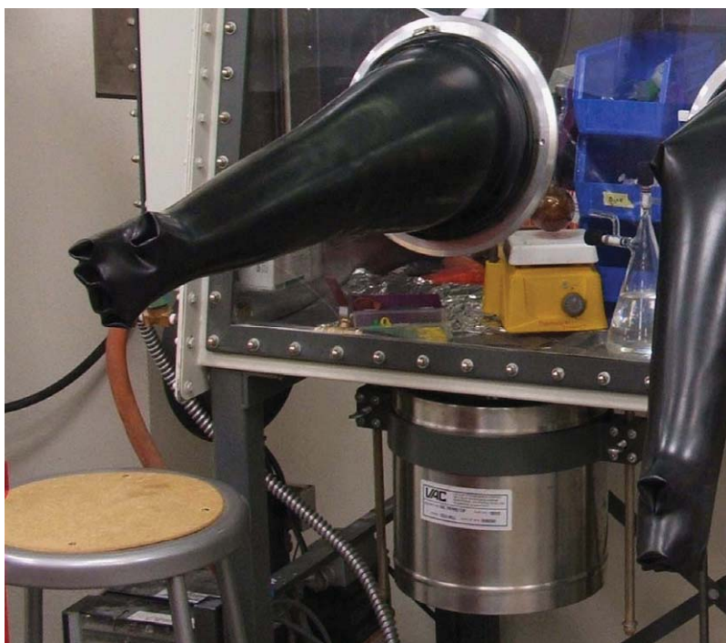
Figure 20 Picture of a Vacuum Atmospheres Co. (VAC) glovebox equipped with a cold well.
