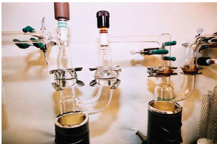
Figure 3 Two solvent traps in series. The left trap is connected to the manifold by O-ring joints while the right trap is connected through ball and socket joints.
