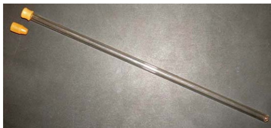
Figure 16 An NMR tube fitted with a small rubber septum.
