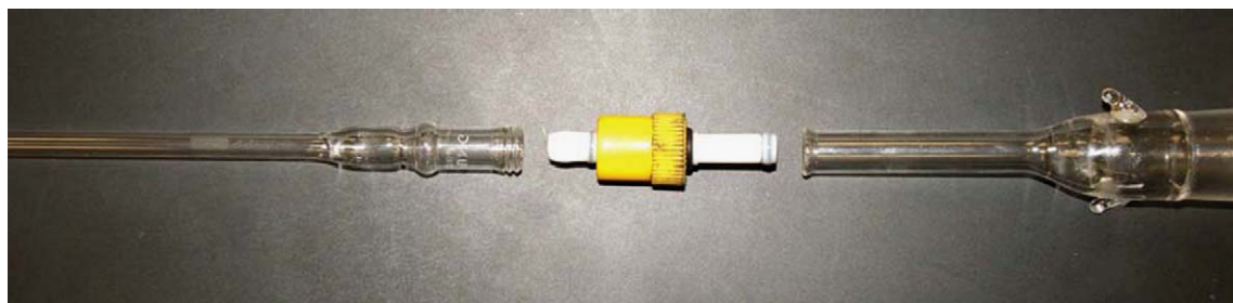
Figure 13 Top of a J. Young NMR tube (left), a J. Young valve (center), and a manifold adapter for a J. Young NMR tube (right).
