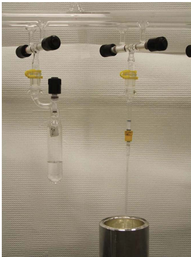
Figure 18 Typical setup for transferring deuterated solvents on a high vacuum manifold.
