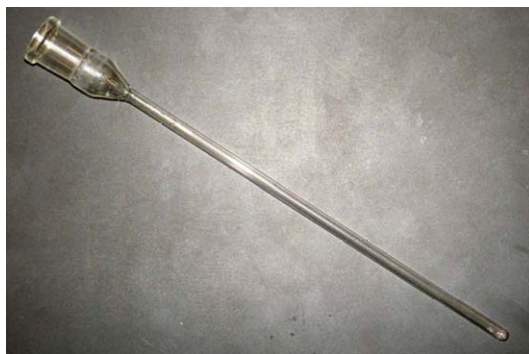
Figure 14 An NMR tube blown to a standard taper ground-glass joint.
