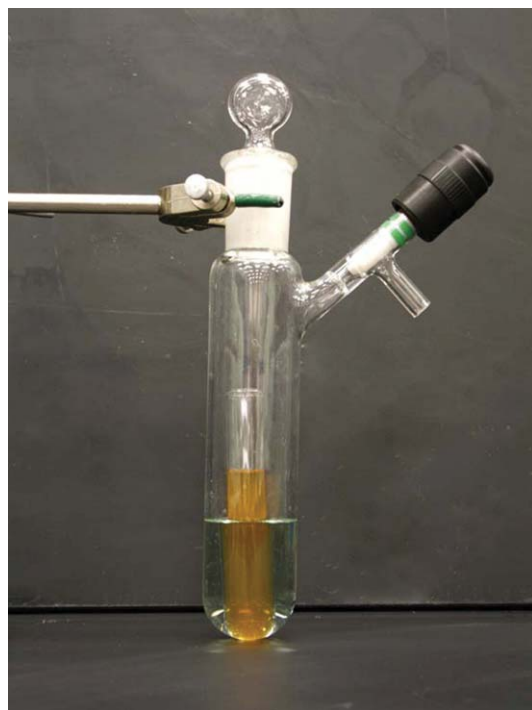
Figure 11 Picture of a vapor diffusion setup for crystal growth inside a Schlenk tube. Solvents are colored for better visual aid.
