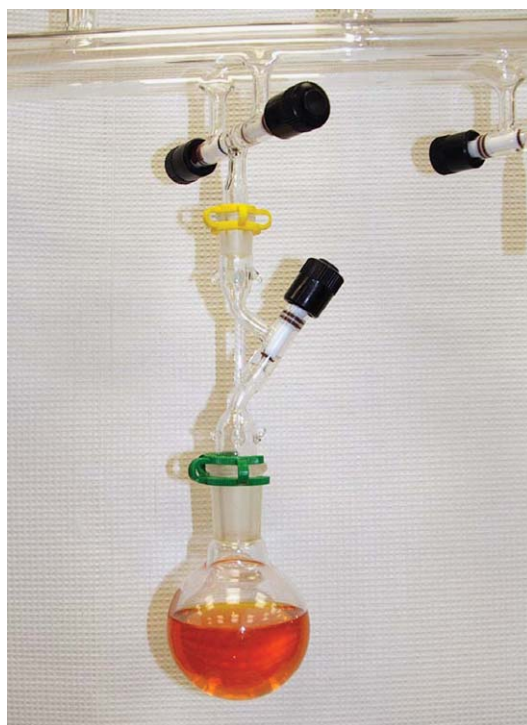
Figure 6 A round bottom flask fitted with an adaptor and attached to a high vacuum line.
