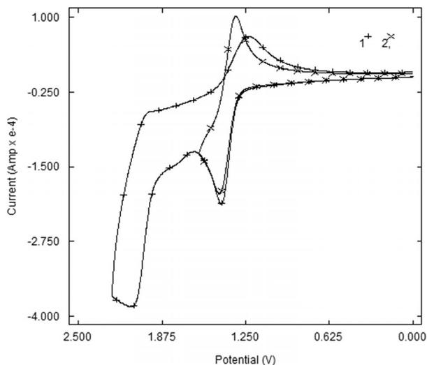
Figure 3. Cyclic voltammogram of 10<sup>-2</sup> M [Ni(BF<sub>4</sub>)<sub>2</sub>(bpy)<sub>3</sub>] in MeCN with the use of a glassy carbon electrode, 10<sup>-1</sup> M [NBu<sub>4</sub>][PF<sub>6</sub>] as supporting electrolyte, at a scan rate of 100 mV/s; reference electrode Ag/AgCl.
