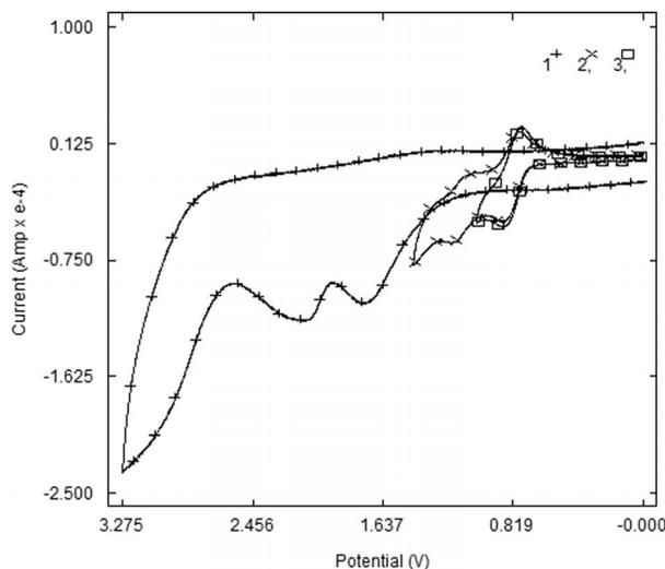
Figure 1. Cyclic voltammogram of 10<sup>-2</sup> M Pd(OAc)<sub>2</sub> (curve 1) and a mixture of Pd(OAc)<sub>2</sub> and 10<sup>-2</sup> M PhPy (1:1) (curves 2 and 3) in CH<sub>2</sub>Cl<sub>2</sub> with the use of a glassy carbon electrode, 10<sup>-1</sup> M [NBu<sub>4</sub>][PF<sub>6</sub>] as supporting electrolyte, at a scan rate of 100 mV/s; reference electrode Ag/AgCl.
