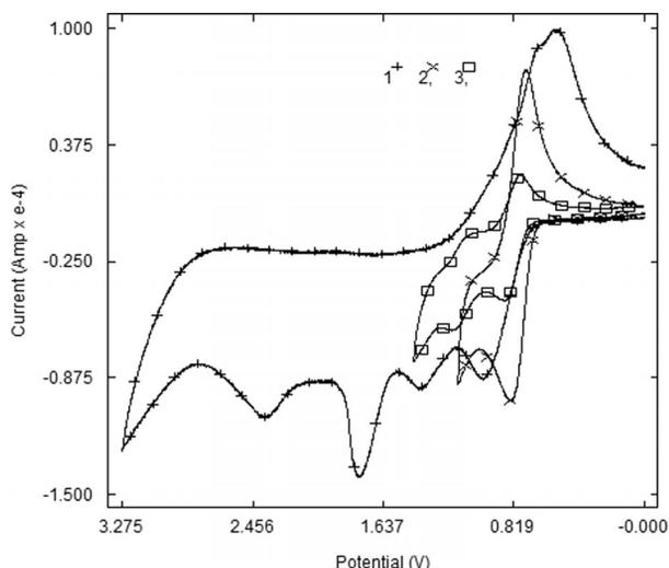
Figure 2. Cyclic voltammogram of 10<sup>-2</sup> M Pd<sub>2</sub>(PhPy)<sub>2</sub>(OAc)<sub>2</sub> (curves 1 and 2) and a mixture of Pd(OAc)<sub>2</sub> and 10<sup>-2</sup> M PhPy (1:1) (curve 3) in CH<sub>2</sub>Cl<sub>2</sub> with the use of a glassy carbon electrode, 10<sup>-1</sup> M [NBu<sub>4</sub>][PF<sub>6</sub>] as supporting electrolyte, at a scan rate of 100 mV/s; reference electrode Ag/AgCl.
